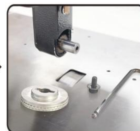
Change the flower wheel, and mount the flower wheel, shim and screw in turn
